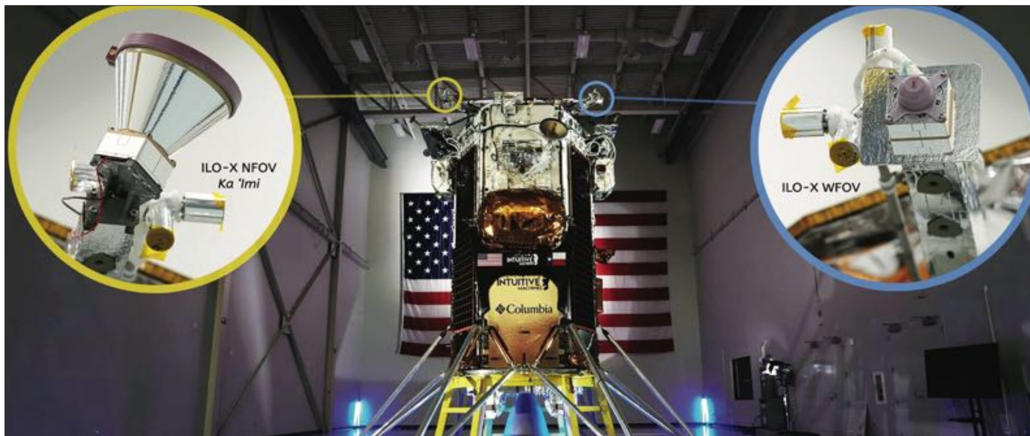
The Canadensys Near Field of View (NFOV) and Wide Field of View (WFOV) optical instruments designed and built for the ILO-X mission are mounted on top of the IM-1 Lunar Lander, which has just arrived at the NASA Kennedy Space Center and is being prepared for launch. CONTRIBUTED PHOTO
