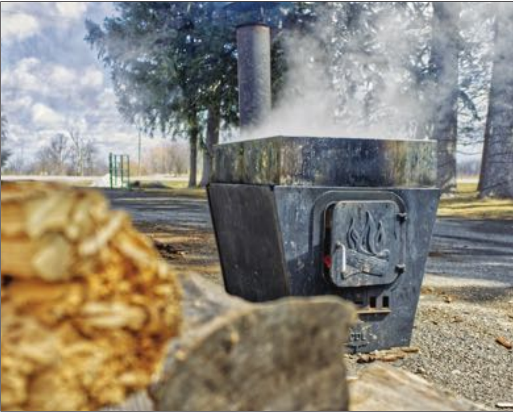
Pigeon uses this evaporator pan to boil sap as part of his maple-syrup making process. PHOTO BY ZACHARY ROMAN
