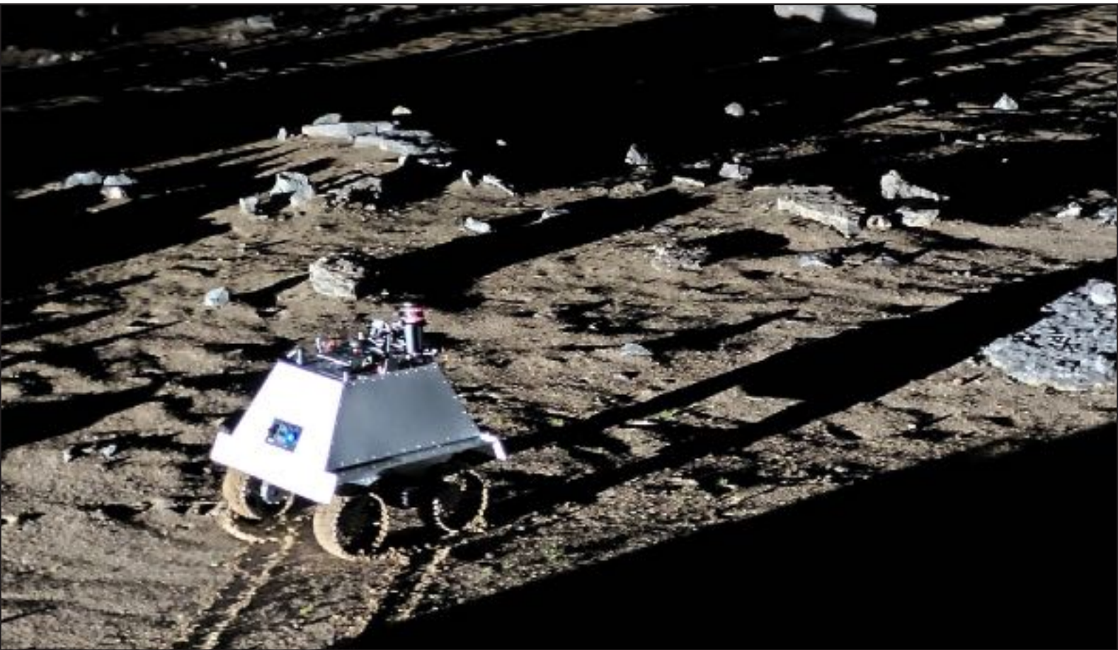
BOLTON FIRM TESTING LUNAR EQUIPMENT: Bolton-based Canadensys Aerospace Corporation has had a team of guidance, navigation and control engineers and scientists at the Canadian Space Agency/Agence spatiale canadienne’s outdoor planetary test facility in St-Hubert, QC. The company designed a terrestrial carrier vehicle to put its lunar navigation sensors and system to the test. “We’re excited to be working closely with our Canadian Space Agency/Agence spatiale canadienne and NGC Aerospace colleagues on this test campaign, which brings us one step closer to having our rover operating on the Moon,” the company says.
