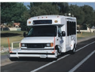
This is the RST, a one-tonne Ford van with high-quality cameras, GPS receivers and a modified front bumper which contains sensitive electronic equipment.
